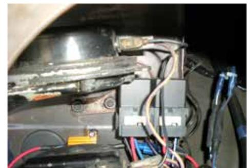
*Michael placed the relays controlling his headlights adjacent to the horns, hidden behind the left outer headlight. Another part of Michael's electrical project was to add a relay to the relay panel so that the headlights only have power when the key is turned on. The gold resistor visible just above the lower horn is for daytime running lights.*
